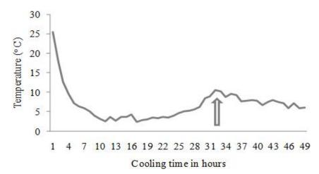
Fig. 1: Curve of temperature inside the Botutainer<sup>®</sup>; the arrow indicates the moment of replacement of the recyclable ice.
